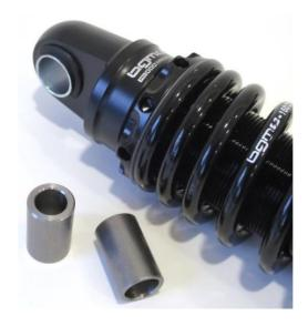
On Luna Line scooters, when converting to a taller (100cc, 125cc or **CPOne35**) cylinder, the (taller type) cylinder cowling comes into close proximity to the underside of the frame and under heavy suspension movement, these can come into contact. To eliminate this, we suggest the use of a <u>BGM Lambretta rear shocker</u> for a Series 3/ GP-DL with <u>two special reduction bushes</u> that **Casa Performance** manufacture.
