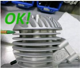
11. Fit the cylinder head onto the cylinder and ensure it is fully seated home.
