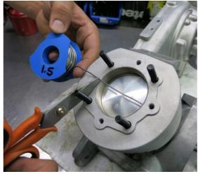
10. With the piston in a position slightly back down into the cylinder i.e. <u>NOT</u> at top dead centre ('TDC'), place a 6cm length of solder (that is preferably 1.5mm thick) on top of the piston crown, along a line that corresponds with the gudgeon pin, as per the photo above.
