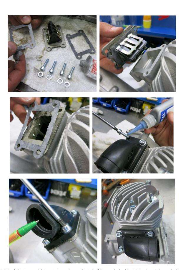
16. Carefully place an inlet gasket over the reed petals of the reedvalve block. Then insert the reedvalve into the cylinder. Place the second inlet gasket on top of the reedvalve. Then mount the rubber inlet manifold. Apply a small drop of medium strength Loctite threadlock (or similar) to the 4 x Allen screws. Add their flat 6mm washers and tighten the whole reedvalve assembly to the cylinder.
