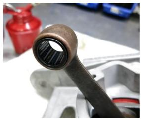
4. Add a drop of 2-stroke oil to a new small end bearing and slide it into the conrod. The **CPOne35** piston is designed to be used with a standard largeframe Lambretta 16x20x20 size small end bearing.
