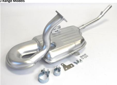
Casa Performance manufactures a standard-type Maxibox exhaust for J Range models. Power output for a CPOne35 engine fitted with a Maxibox exhaust should produce at least 10bhp when combined with an out-of-the-box CPOne35 kit, in completely untuned format. This is the dedicated exhaust for use with the kit (see above pic), and the use of any other exhaust could seriously compromise the power output of the kit.
