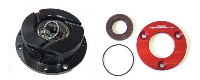
**Casa Performance** has also manufactured a CNC machined drive side <u>oilseal plate</u> (above right). This has an additional **Viton O-Ring** and offers perfect sealing, and comes ready supplied with a Viton oilseal (with a choice of oilseal for either 3-speed and 4-speed casings).
