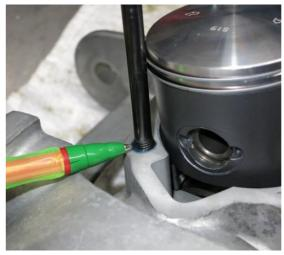
6. If you have previously removed short 50/75cc type cylinder studs, now fit the longer type cylinder studs, applying a small drop of medium strength Loctite threadlock (or similar) to the threaded sections that will be inserted into your engine casing. Once fully fitted, clean off any excess Loctite from around the bottom of each stud.
