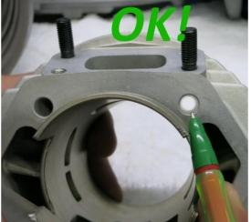
7. Fit the 4 exhaust studs, applying a small drop of medium strength Loctite threadlock (or similar) to the SHORTER threaded sections, that will be inserted into the cylinder.
