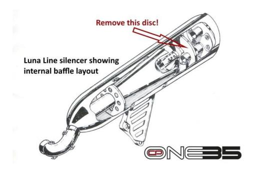
If you use an original type Vega 75cc model exhaust, power output will be approx. 10bhp at the rear wheel, and if you modify that same exhaust by removing a 'baffle' disc (as seen in the 60's Lambretta Tuning Manual), you'll see an extra 10% power.
