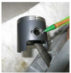
5. Fit both piston rings to the piston and then <u>one</u> circlip. We thoroughly recommend the use of the 16mm version <u>circlip fitting tool</u> when doing so that have made manufactured. This superb tool makes exceptionally light work of a difficult job as can be seen in <u>this YouTube video</u>.
