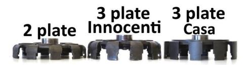
The clutch spiders have two different sizes of the central splined hole, which is either SMALL or LARGE, where it fits onto the gearbox cluster. When choosing a clutch spider for your scooter, ensure it is a **3-plate type** with the correct sized central splined hole to match your gearbox cluster.
