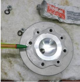
15. Apply a smear of <u>Threebond sealant</u> to the machined 'gasket face' area of the cylinder head, and allow it a little drying time. Fit the cylinder head onto the cylinder and ensure its fully seated home. Again, take care to ensure that the cylinder head is correctly seated inside the cylinder!
