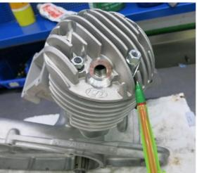
Tighten each nut slightly, in a criss-cross diagonal fashion, as per the sequence of the **red** numbers in the photo above, until all four are tightened up to **15Nm**. Fit the split and flat washers to the 3 x 6mm Allen screws and fit them to the cylinder head. Tighten them up fully to **11Nm** as per the sequence of the **green** numbers in the photo above. Turn the crankshaft by hand to ensure the engine rotates smoothly.
