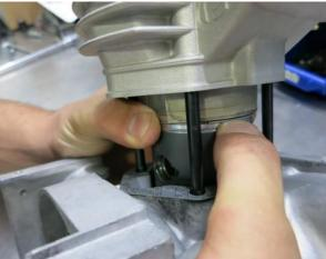
9. Now you need to slide the cylinder down over the studs, until it comes into contact with the top of the piston. Gently squeeze each piston ring to close it up, to allow the cylinder to drop down over the piston. Once both piston rings are inside the cylinder, gently slide it downwards until it's fully seated home on the engine casing. Now turn the crankshaft by hand to ensure the piston can travel freely within the cylinder.
