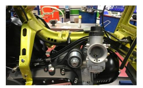
One of the biggest problems with scooters having a right-hand (kickstart side) exiting carburettor is that it can easily come into contact with the scooters control cables. If these same cables come into contact – even minimally – with the carburettor (especially under suspension movement), then the chances are that this will cause the failure of the carb rubber manifold in a short space of time. If you are unsure the outer
