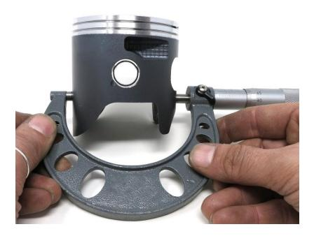
When measuring your piston, a Micrometre MUST be used (a digital vernier is NOT acceptable) and the measurement taken exclusively at the point as seen in the photo above.
